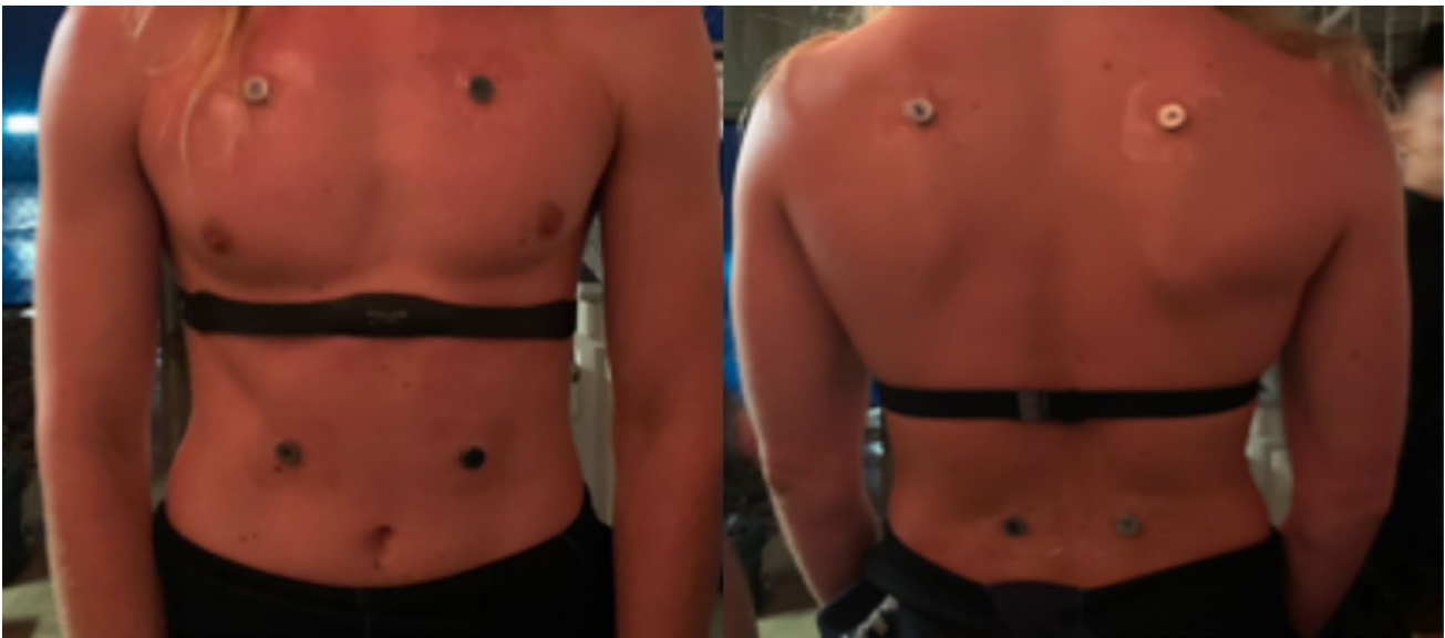
Fig. 2 Image of thermistor and heart rate transmitter placement for laboratory study
